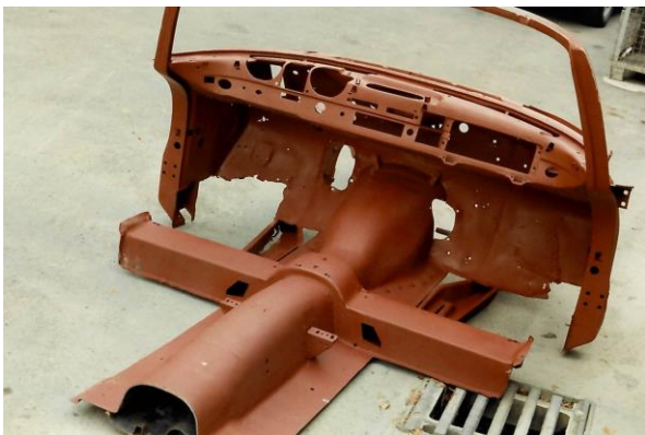
This pre-restoration condition shows where and to what extent metal sheets had to be fitted for the restoration (above and below)
