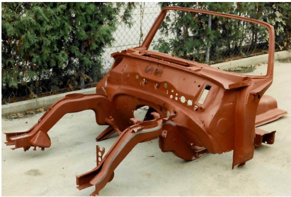
This pre-restoration condition shows where and to what extent metal sheets had to be fitted for the restoration (above and below)
