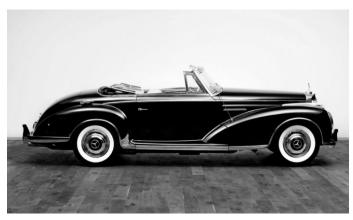
unchanged. But thanks to the new direct petrol injection system – as in the sporty 300 SL – the engine now delivered 175 hp. The sophisticated injection system was the highlight of series production and was emphasised with an EINSPRITZMOTOR (injection engine) engraving on the rear bumper. Like the 300c sedan, the chassis had a single-joint swing axle with a low pivot point for significantly better road holding.
