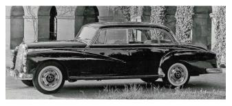
had mechanical intake manifold injection with an output of 160 hp. Moreover, an automatic gearbox was standard, but a manual transmission was available as an alternative on request. From March 1958, power steering was available as an option, but this was reserved for vehicles with automatic transmission.
