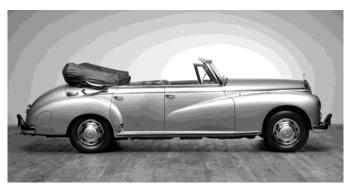
The 300c was the revised version of the 300 from 1955 and had the internal designation W186 IV. The main innovation was the modernised single-jointed rear axle, which provided significantly better road holding. In addition, the final expansion stage of the 300 carburettor engine with 125 hp instead of 115 hp had a powerful effect. Visually, the 300c can be recognised by the hinged windows in the
