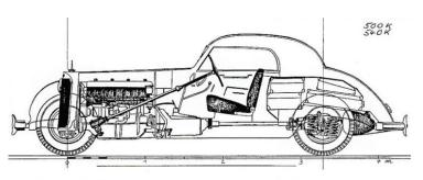
required a new crankshaft. A high-speed gearbox with semi-automatic shifting was used for the 500 K transmission. The clutch did not need to be operated when shifting from third (direct) gear to high gear.
