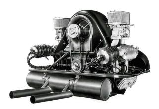
In 1955, the sports version of the 356 A, the 1500 GS (Gran Sport) or Carrera, was launched. Its engine was based on the high-performance engine newly developed in 1953 for the legendary 550 Spyder racing car. The engine by Porsche engineer Ernst Fuhrmann uses four overhead camshafts for the four-cylinder boxer engine (type 547), which is only 1.5 litres in size, and is driven via king shafts for high speed stability and exact adherence to the valve timing. This thoroughbred racing engine with
