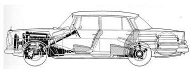
Instead of carburettors, the engine of the 220 SEb had a mechanical intake manifold injection system from Bosch (twin-ram injection pump) and an output of 120 hp.
