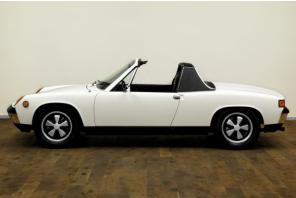
At its launch, the 914 was available with two engine options. The 914 with 1.7-litre four-cylinder boxer engine and 80 hp from Volkswagen as well as the 914/6 with a 2.0-litre six-cylinder boxer engine and 110 hp from the Porsche 911 T.
