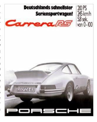
The distinctive rear wing, nicknamed the "duck-tail", significantly improved driving stability. The special front spoiler had an opening in the middle for an oil cooler. Differently wide wheels on the front and rear axles ensured higher cornering speeds and stronger braking performance. In the rear axle area, the body is 42 millimetres wider.
