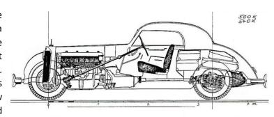
gearbox with semi-automatic shifting was used for the 500 K transmission. The clutch did not need to be operated when shifting from third (direct) gear to high gear.
